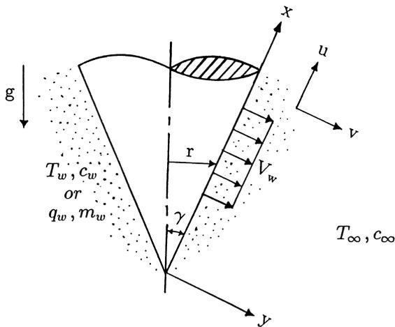
Fig. 1. Flow model and physical coordinate system.
